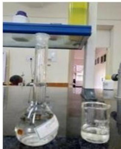
Fig1:4.75g(100ml)Cerium nitrate And 1.6g(15ml) NaOH solution
