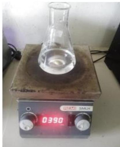
Fig2:Cerium nitrate under stirring at 350rpm
