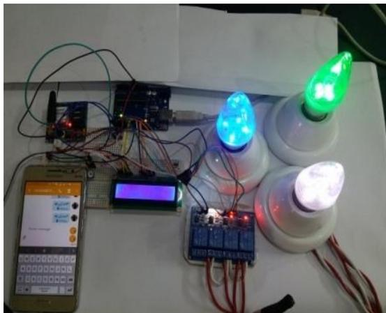
**Fig -6.** Actual GSM Based Home Automation
