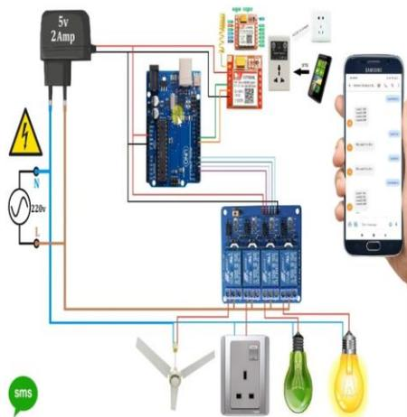
**Fig -5** Block Diagram of GSM Based Home Automation
