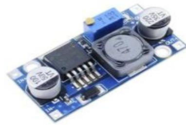
Fig 5: DC to DC Buck Converter
