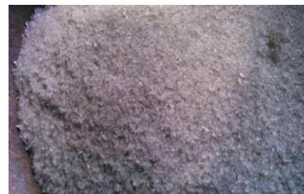
**Fig 4.** Crushed Glass Powder
