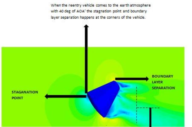
When the reentry vehicle comes to the earth atmosphere with 40 deg of AOA' the stagnation point and boundary layer separation happens at the corners of the vehicle.
