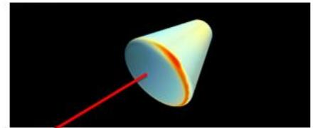
According to the definition, the ablative heat shield's blunt body has the maximum rate of heat conduction when descending at 40 degrees
