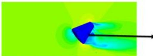
FIG 5: VELOCITY CONTOUR OF 40 AOA'
