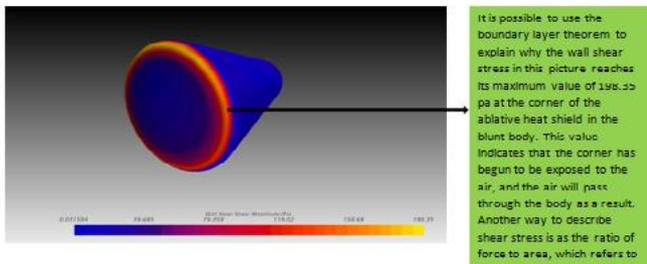
**FIG 14: WALL SHEAR STRESS CONTOUR OF 18 DEG AOA'**
