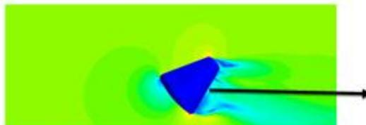
FIG 6: VELOCITY CONTOUR OF 40 AOA'
