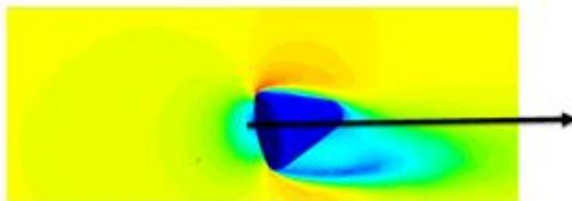
FIG 4: VELOCITY CONTOUR OF 15 AOA'
