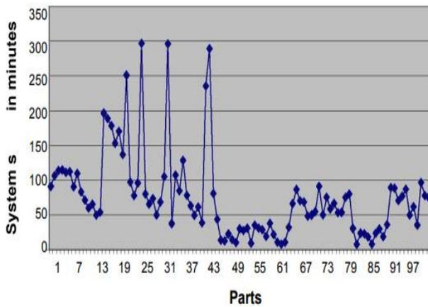
Figure 5.3 Time in system for parts under the LPT scenario
