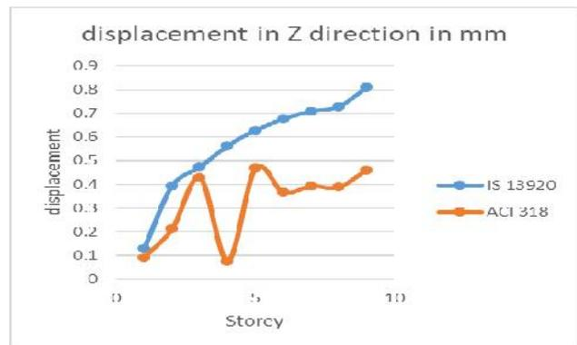
Graph 6.6: Displacement in z direction in mm
