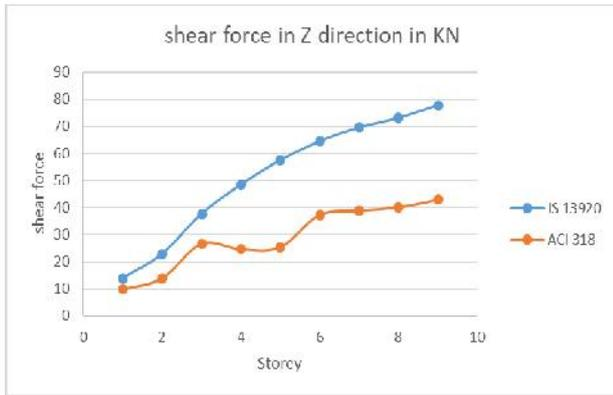
**Graph 6.10: Shear force in Z direction in KN**
