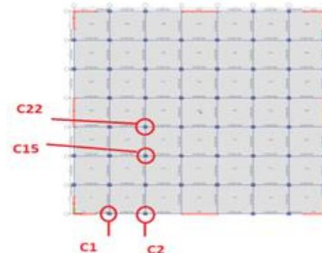
Figure 4(a): Column removal cases for Model A
