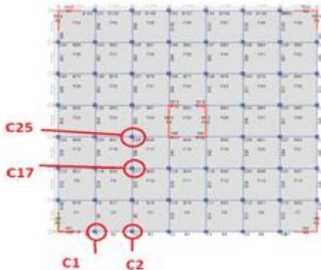
Figure 4(b): Column removal cases for Model B
