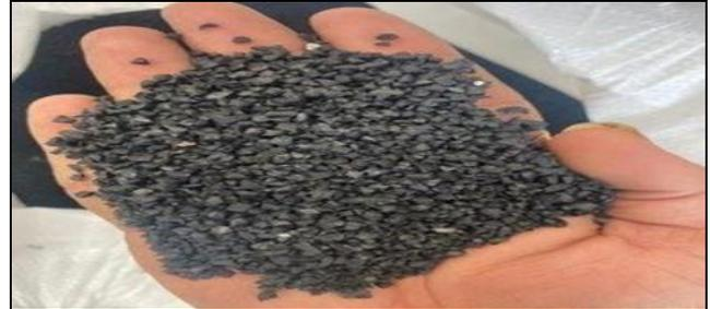
**Figure 2: Waste Shredded Rubber Tyres**
