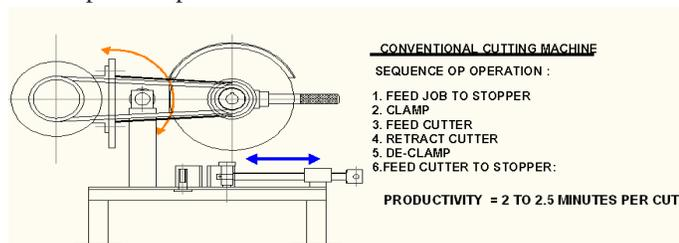
Figure 01: Conventional Cutting Machine
