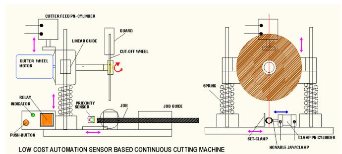
Figure 04: 2d Design of Semi-Automated Robotic System
