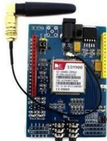
Figure 3: GSM sensor
