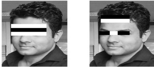
Figure 3: Several Haar-like-features matched to the features of face
