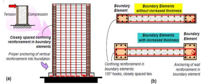
Figure 1: Layout of Main Reinforcement in Shear Wall as per IS:13920:1993
