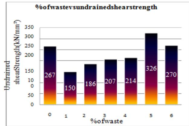
Fig4.4:% of waste vs maximum undrained shear strength.
