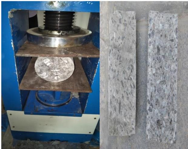
The split tensile strength of the cylinders after addition of fibers with SCC0, SFRSCC2C, SFRSCC2H, HFRSCC (0.5C + 1.5H), HFRSCC (1.0C+1.0H) and HFRSCC (1.5C+0.5H) is studied for 7 & 28days shown in Table 4 & 5.
