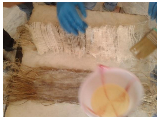
Figure 3.1 Okra-Epoxy Composite Specimen Preparation
