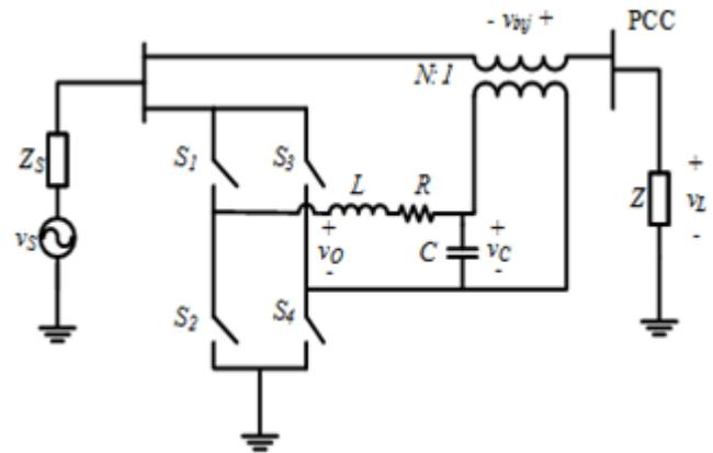
Figure 1. Single-line diagram of AVC
