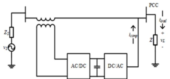
Figure 3. Single-line diagram of APC
