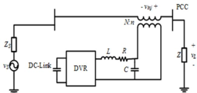
Figure 2. Single-line diagram of DVR
