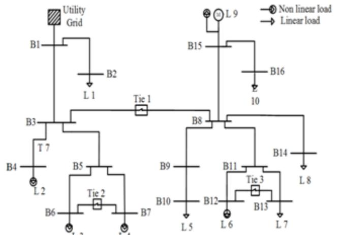
Figure 5. Single-line diagram of the 16-bus test system
