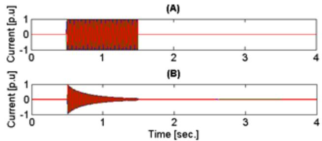
Figure 8. Injected currents during a 0.6 voltage sag and voltage interruption, (A) APC current. (B) D-STATCOM current
