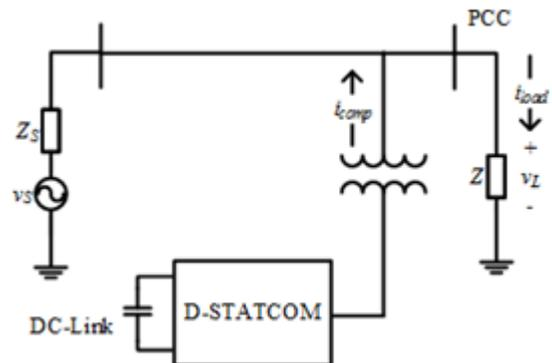
Figure 4. Single-line diagram of D-STATCOM
