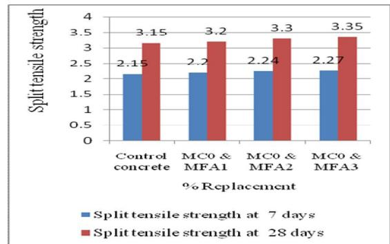
Fig -5 Split tensile strength Vs Mix -I
