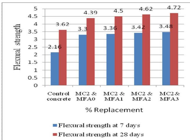
Fig 12 Flexural strength Vs Mix -IV
