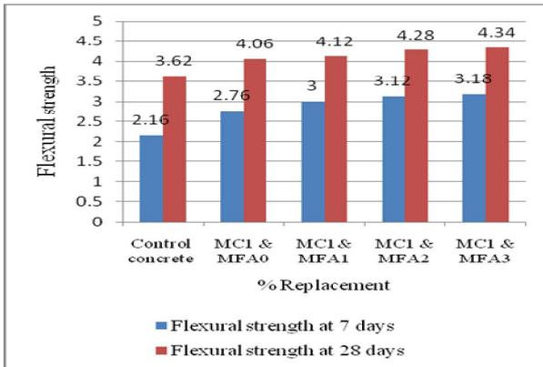
Fig 11. Flexural strength Vs Mix -III
