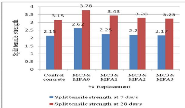
Fig 8 Split tensile strength Vs Mix - IV
