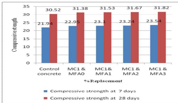
Fig -2 Compressive strength Vs Mix -II
