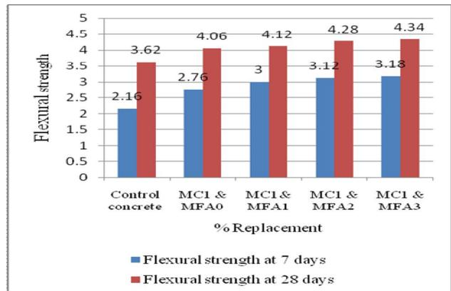
Fig 10 Flexural strength Vs Mix -II
