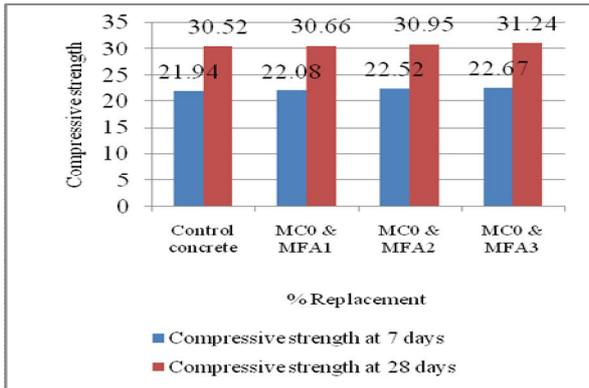
Fig 1- Compressive strength Vs Mix -I
