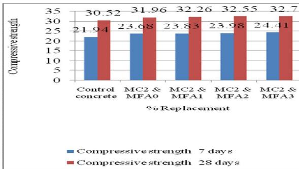
Fig -3 Compressive strength Vs Mix -III
