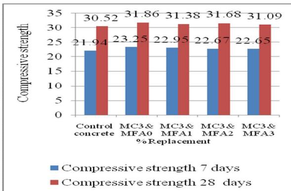
Fig -4 Compressive strength Vs Mix -IV
