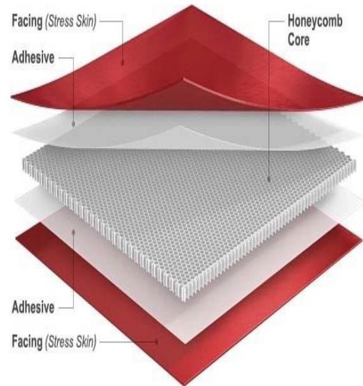
Fig. 1 Descriptive view of a Composite Sandwich Structure
