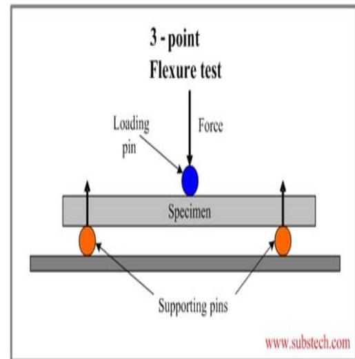
Fig. 4 3-Point Bending Test Setup
