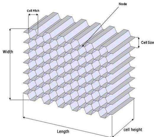
Fig. 2 Honeycomb Structure
