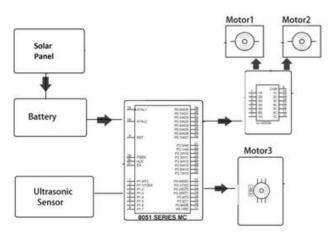
Fig Block Diagram
