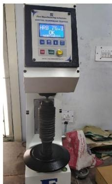
Figure 2.4 Rockwell Hardness testing machine
