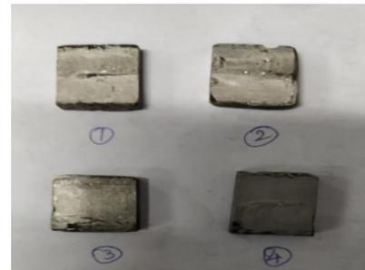
**Figure 2.3 Prepared samples for Hardness test, Microstructural analysis and AFM**
