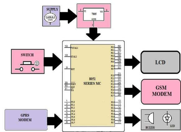
Fig. 9: Circuit diagram of Boat Engine controlling system
