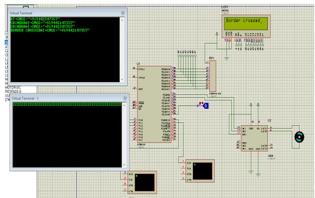
Fig. 13: 8051 with RFID – Crossed the border (Engine OFF)
