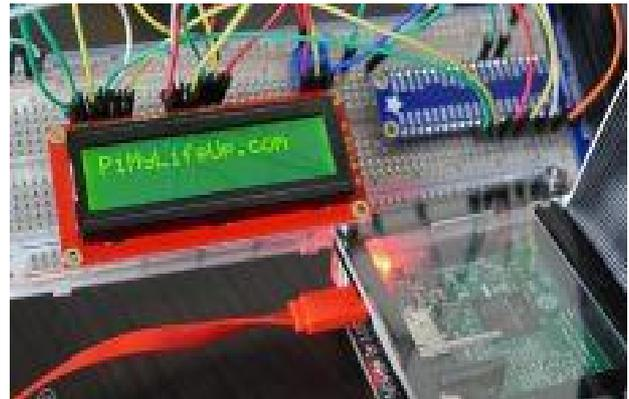
Fig 8. RFID & LCD - Raspberry pi via USB port
