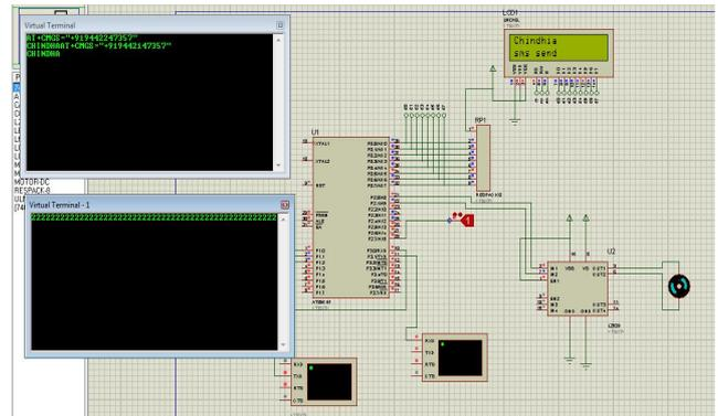
Fig. 12: 8051 with RFID – Boat is with in the Layer (Engine ON)
