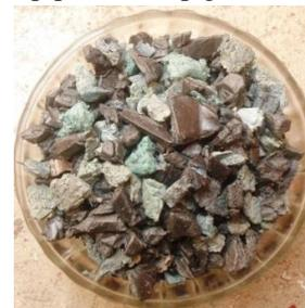
Fig. 2 Combined Recycled Granules of HDPE and LLDPE Pipe Materials
