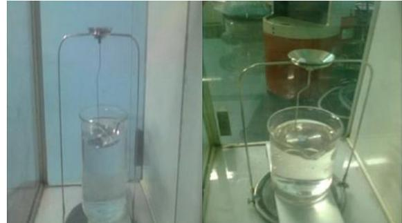
Fig. 11 Displacement method test for measuring the Density
