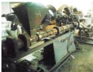
Fig. 1 Typical Conventional Extrusion Line
