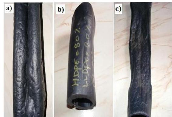
Fig. 10 Bad pipe profiles Extruded at 86°C
