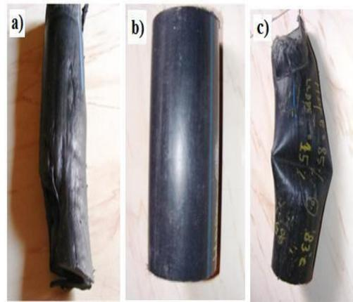
Fig. 9a) and c) shows the bad pipe profiles extruded at 83°C and the fig. b) shows the extruded a better pipe profile.
