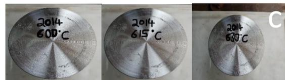
Fig. 4 Thixocast Alloy (a) Before Machining (b) After Machining (c) After Machining ( at diff. processing temperatures)
