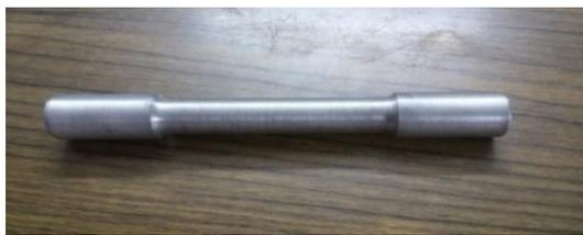
Fig. 3 Specimen for Tensile Testing
