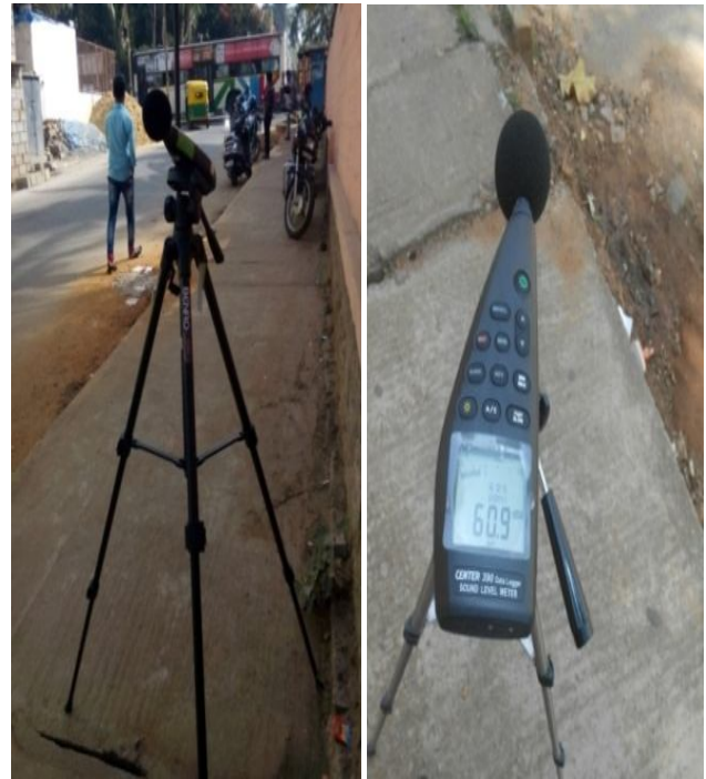
Figure 2: Noise Level Meter apparatus Equipped with Tripod Stand
