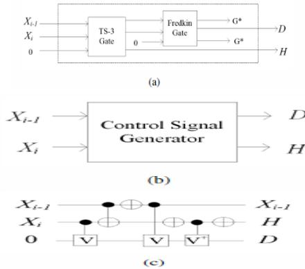
Figure 1. (a) Gates used in 'C' Cell (b) 'C' cell as a block diagram with input and output (c) Quantum circuit for 'C' cell, where QC is 4
