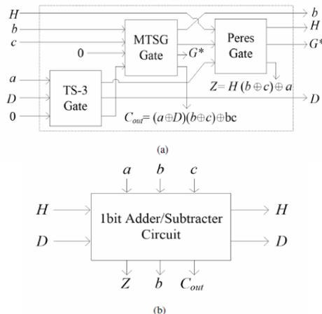
Figure 2. (a) Circuit diagram of B cell (G\* indicates the garbage output) (b) Block diagram of B cell
