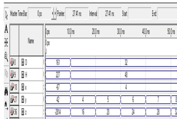
The above figure is Simulation Results for 8 bit booth multiplier. When  $X=42(00101010)$ ,  $Y=-67(10111101)$  signals are given to 8 bit multiplier the output of multiplier generates 2's complement output is  $-2814(0000\ 1010\ 1111\ 1110)$ .
