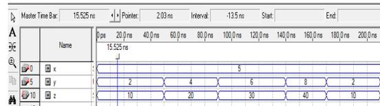
Figure 8. Simulation Results for 4 bit booth multiplier using TSG gate
