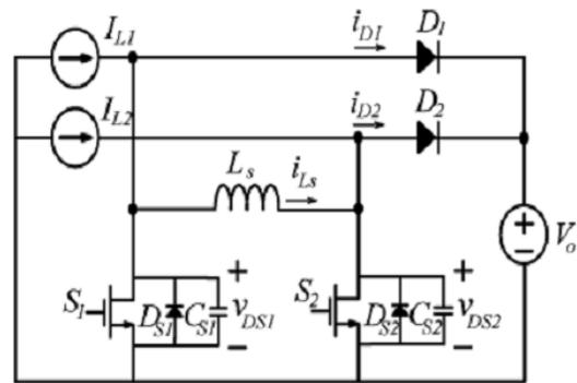
Fig 2. Soft switching converter module
