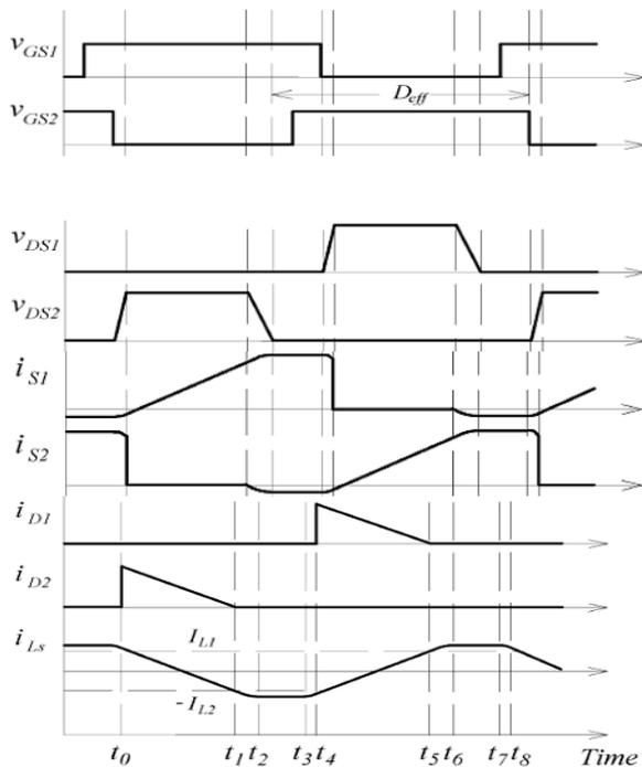
Fig.3. waveforms of Boost Converter
