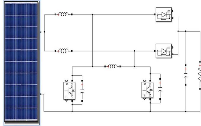
Fig.5. Simulink model of an Efficient Boost Converter
