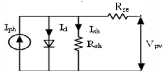
Fig.1. Equivalent Circuit for a Solar Cell
