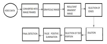
Fig 1 Block Diagram for Text Detection in Video
