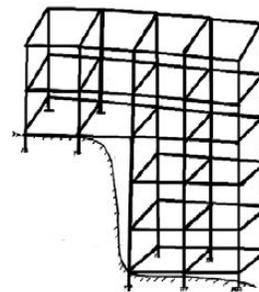
Figure 2.2. Building configurations at vertical cuts/steep slopes
