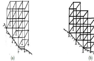
Figure 2.1. Hill building configurations: (a) Step back building; (b) Set back and Step back building
