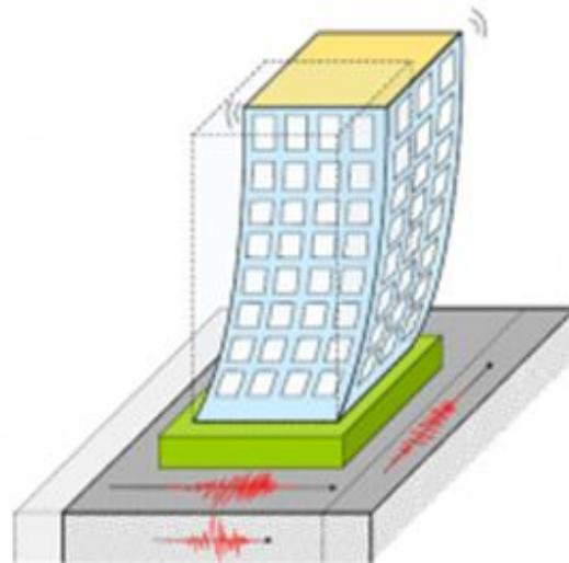
Figure –Behavior of building under earth quake
