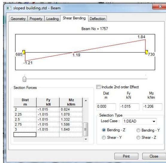
Fig: Column Share force bending moment diagram
