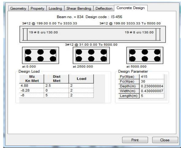
Fig: Beam Concrete Detailing
