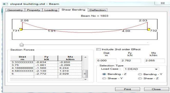
Fig: Beam Share force bending moment diagram
