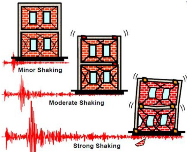
Figure –performance objectives under different intensities of earthquake
