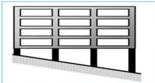
Figure 1: Building frame with short columns
