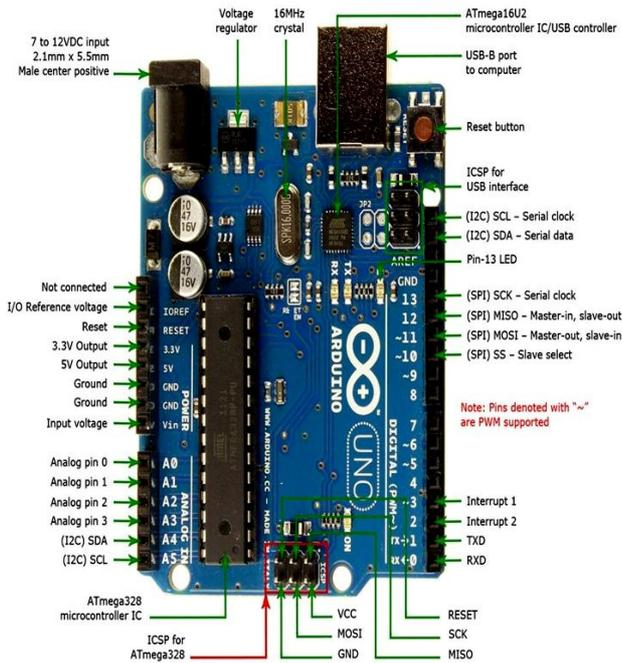
Fig. 2 Arduino Uno Board [11]
