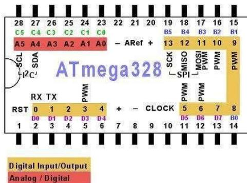
Fig. 3 Pin diagram of ATMEGA328P [11]
