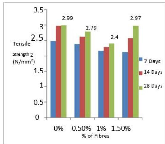
Fig.2. Split Tensile Strength
