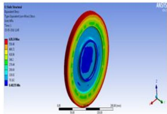
Fig. 14. Equivalent stress of the disk before optimization
