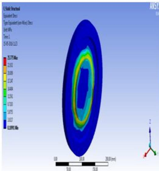
Fig. 10. Equivalent stress of disk subjected to shrink-fitted load
