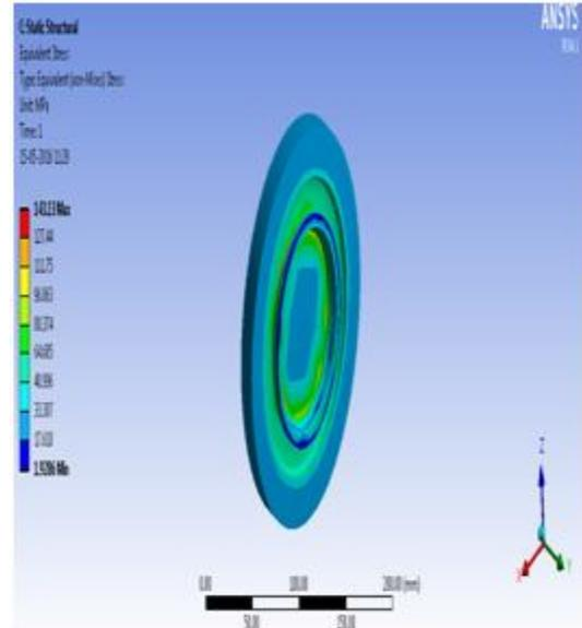
Fig. 11. Equivalent stress of disk subjected to blade load
