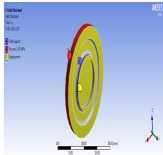
Fig. 6. Disk subjected to blade load
