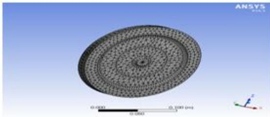
Fig. 3. Fine mesh of disk
