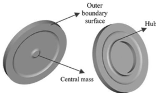
Fig. 1. Gas turbine disk
