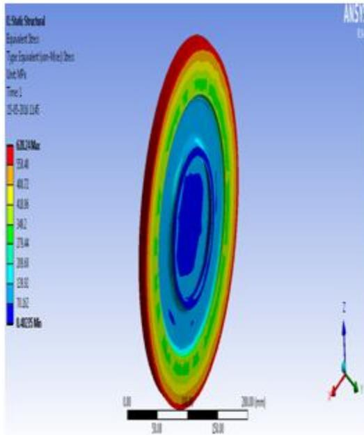
Fig. 13. Equivalent stress of disk subjected to combined load
