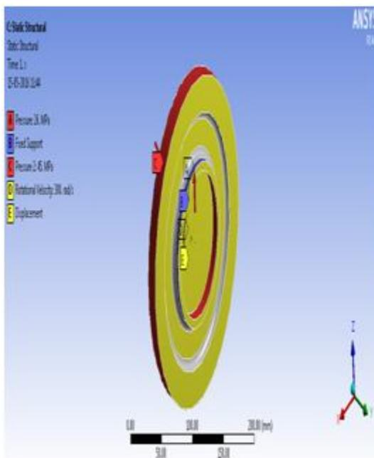
Fig. 8. Disk subjected to combined load
