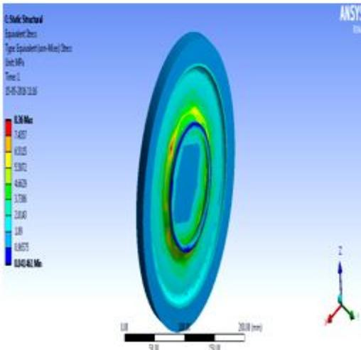
Fig. 9. Equivalent stress of disk subjected to rotational load
