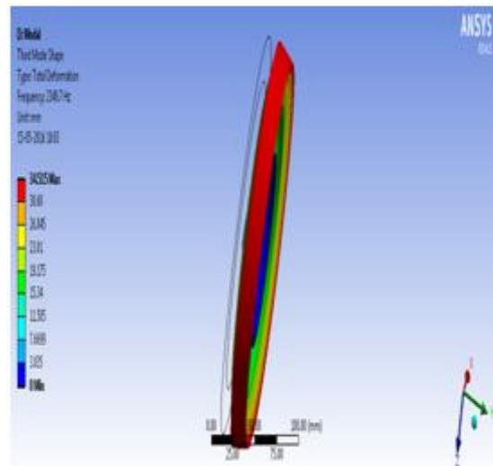
Fig. 18. Mode 3 at 2349.7Hz
