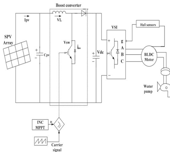
**Fig. 5.1 Configuration of the SPV array fed BLDC motor driven water pumping system.**
