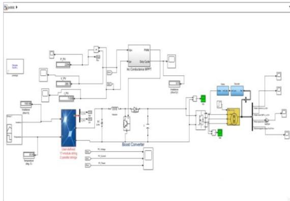
**Fig.7.1 Simulink model for solar powered brushless dc motor drive for water pumping system**
