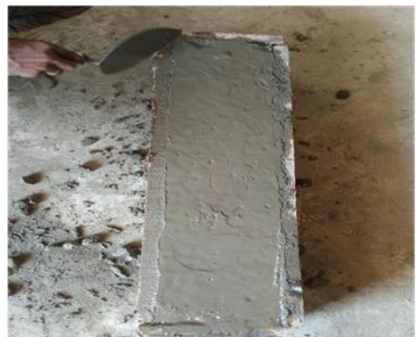
Fig.5. Finishing of Surface
