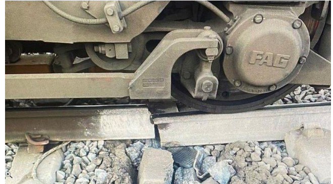
Fig. 1 Part of the track which was completely broken
