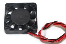
5V DC fan is a compact and low-power device that provides cooling and airflow in various electronic applications. Its size, airflow capacity, bearing type, and noise levels can vary, allowing users to select a fan that suits their specific cooling needs while considering factors such as power consumption and space constraints.
