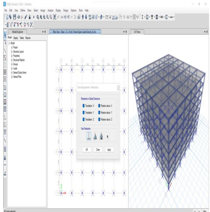
**Fig 6 Assigning Fixed Support**
