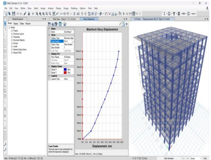
Fig 10 Storey Displacement
