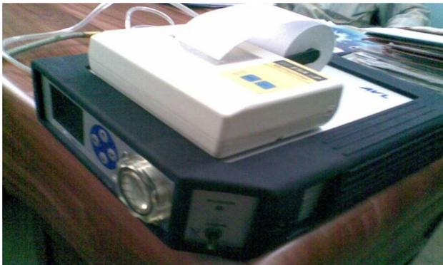
Fig. 3. Emission analyzer (AVL Digas 444).
