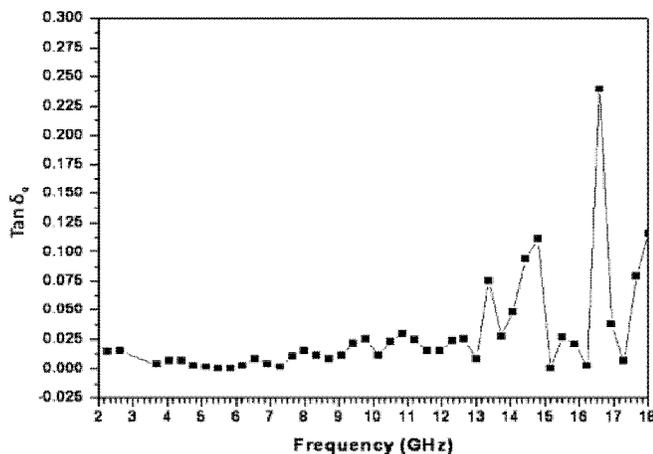
Figure 2: Di-electric tangent loss ( $\tan \delta_e$ ) vs. Frequency (GHz) variation
