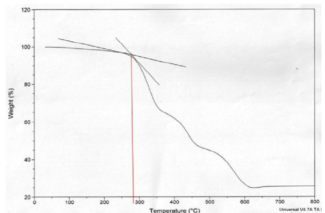
Figure 8: Thermo gravimetric analysis of  $Ni_{0.5}Zn_{0.5}Fe_2O_4$  nano composite
