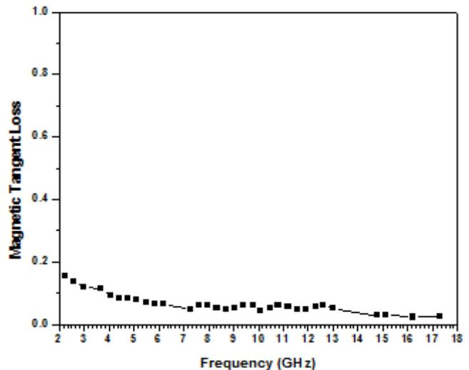
Figure 4: Magnetic tangent loss ( $\tan \delta_m$ ) vs. Frequency variation
