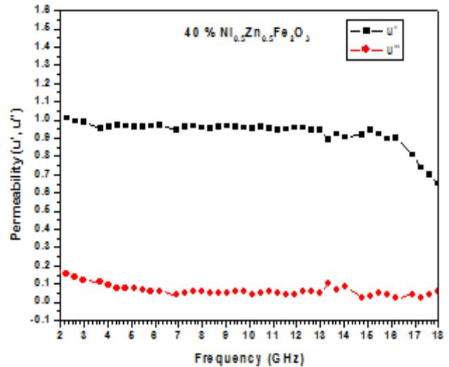
Figure 3: Complex Permeability vs. Frequency (GHz) variation
