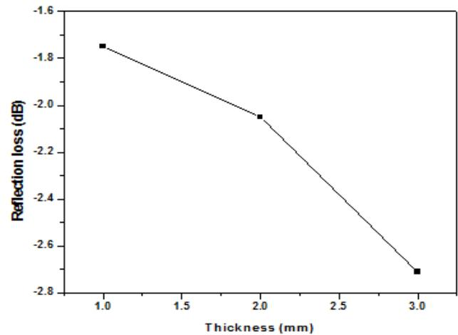
Figure 6: Maximum Reflection loss ( $R_{L, \max}$ ) vs. thickness (mm)
