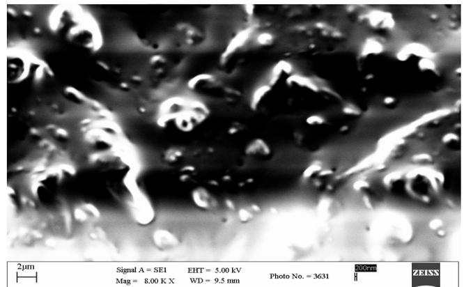
Figure 7: SEM of 40% (by wt.)  $Ni_{0.5}Zn_{0.5}Fe_2O_4$  Nano powder in PU
